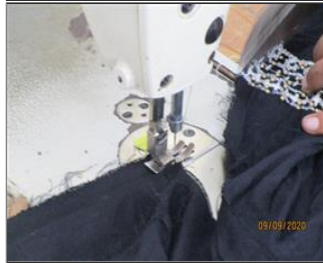
Photo of non-conformity needle guard was not provided.JPG
