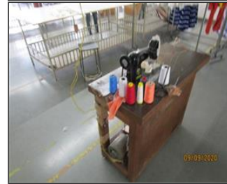
Photo of non-conformity pulley guard was not provided.JPG
